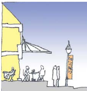
➤ P85: Section showing the relationship between building, ground floor uses, sitting out area, pedestrian and road...an example of an active friendly edge and friendly environment.
