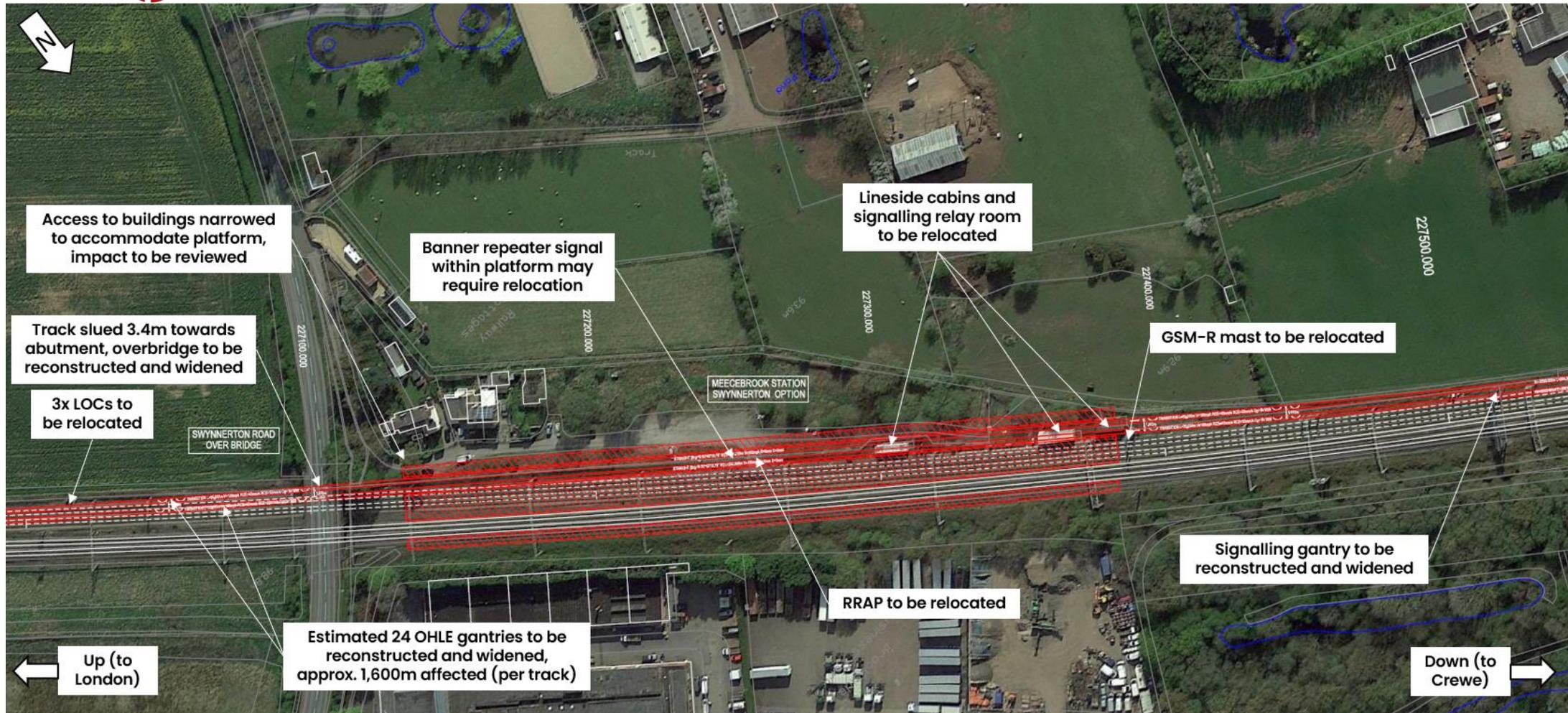
**Figure 6 – Swynnerton Option impact assessment (see Section 5 and Appendix A for detail)**
