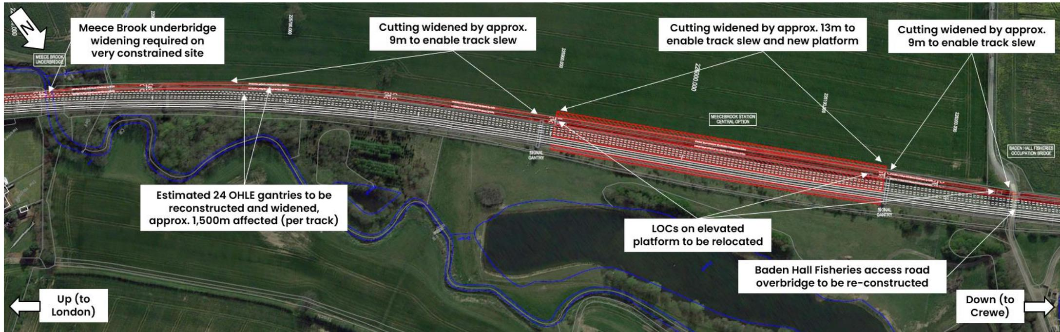
Figure 10 – Central Option impact assessment (see Section 5 and Appendix A for detail)
