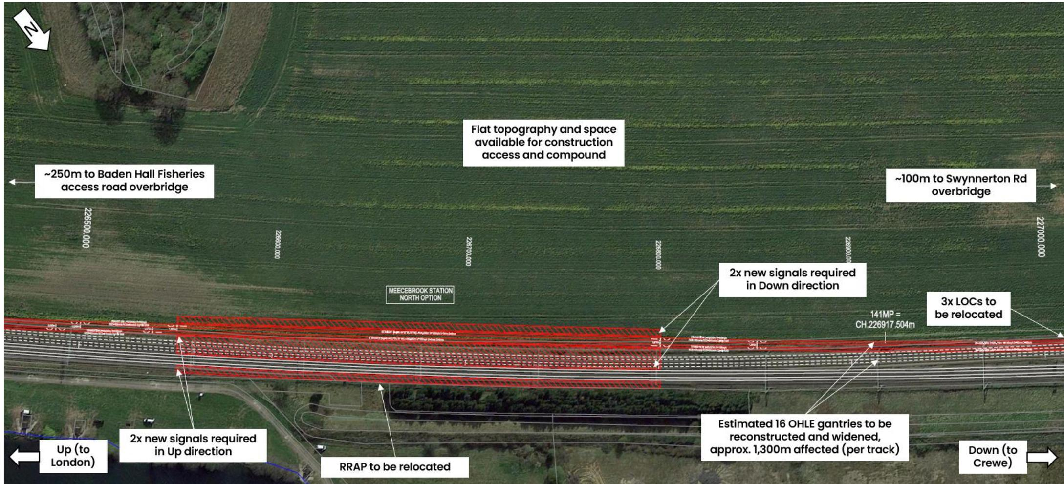
Figure 8 – North Option impact assessment (see Section 5 and Appendix A for detail)
