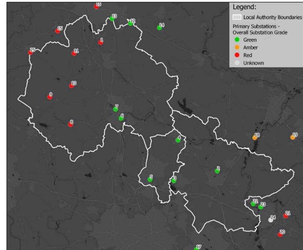
Figure 8—2 RAG analysis to provide an indication of available capacity at the primary substations in the LAEP area. Basemap from ESRI with substation data provided by WPD.
